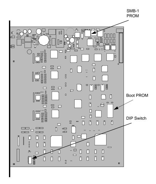
Figure 2-2. User-Accessible Components
